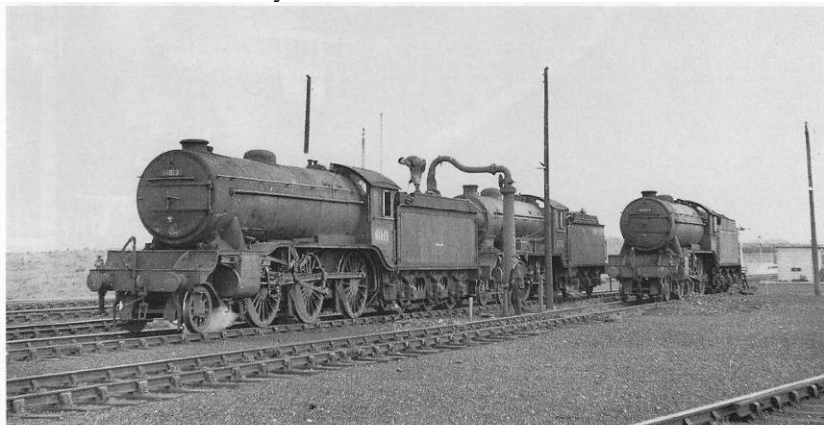
A line-up of Gresley medium-sized steam power at the Camp loco servicing area. Two water cranes and ash pits were provided for servicing engines ready for their return journeys. This picture shows 'K3' No. 61813 of Hull Dalrycoates shed (53A) taking water, coupled to D49/1 No. 62703 Hertfordshire of Bridlington shed (53D). It is likely that the 'Shire' was attached to the K3's train at Bridlington to give assistance over the 5½ mile climb up to Speeton. Three different types of tender can be seen. 'K3' No. 61893 on the right has the LNER group standard type with flat sides, the other 'K3' has the flared top version and the D49 has an ex-NER design behind it.
