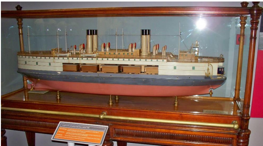
Armstrong-Whitworth model of train-ferry Baikal , Discovery Museum, Newcastle 16/2/24 NB Propellers at both ends, wagons behind cutaway sides, and carriage-end peeping out at right
