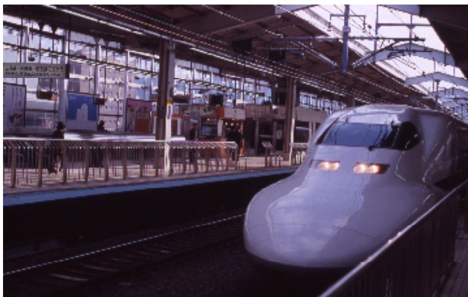
Monday 13 th October 2008 – 08.30 for Hiroshima pulls into Kyoto station. Formation is 16-car "Nozomi" ("Hope") 700-series "bullet train". Note continuous platform barriers except opposite carriage doors. D. Peel
