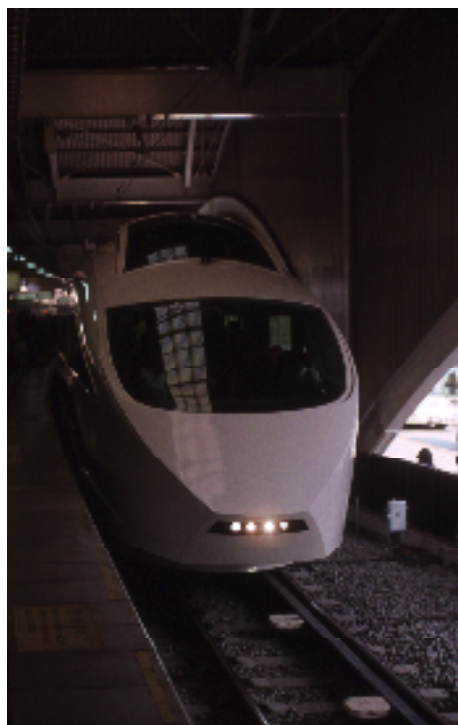
Saturday 18 th October 2008 – 4-car emu entering Yunnoto station on local service (3' 6" gauge). Track on left is 4' 8½" gauge, so rear coaches are running on mixed gauge track D. Peel
