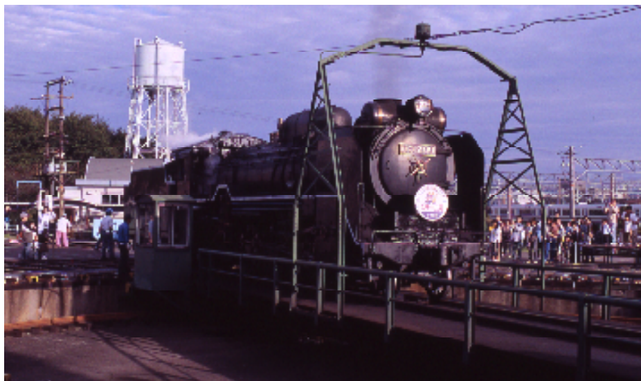
Sunday 12 th October 2008 – Umekoji Working Steam Museum, Kyoto. 2-8-2 class D51 no.200 runs onto the turntable at the end of a day's operating. Most numerous class of all JNR locos, 1115 were built from 1936 onward. 35 were later equipped with Giesl ejectors. (3' 6" gauge) D. Peel
