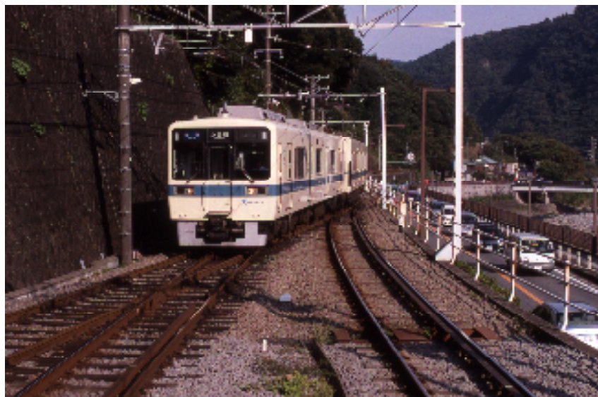
Saturday 18 th October 2008 – 4-car emu entering Yunnoto station on local service (3' 6" gauge). Track on left is 4' 8½" gauge, so rear coaches are running on mixed gauge track D. Peel
