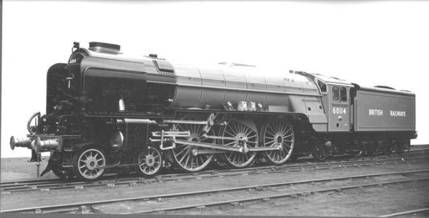
№ 60114, BUILT IN 1948, CLASS A1. DR WH'LS 6' 8". № 525, BUILT IN 1947, CLASS A2. DR WH'LS 6' 2".
