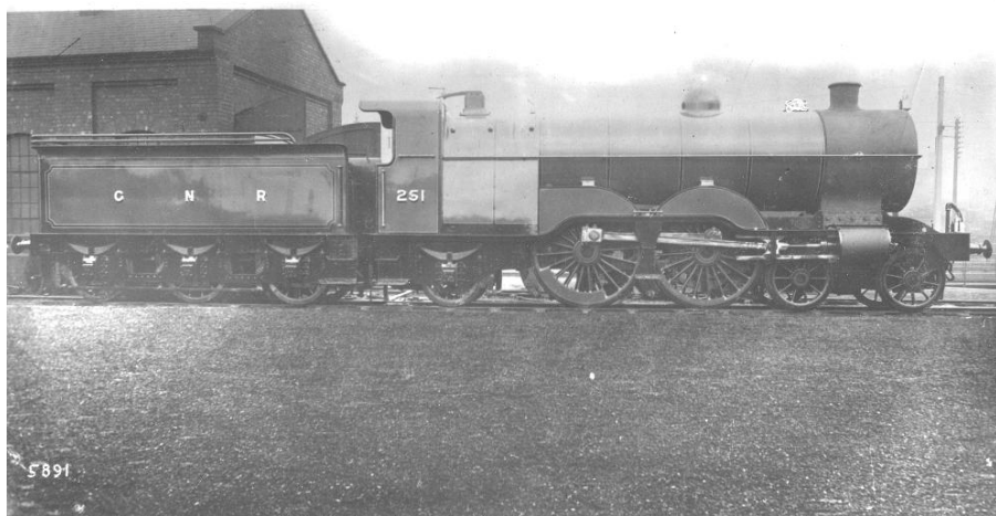
G.N. No 251 AS FITTED WITH STOVEPIPE CHIMNEY IN 1909 (PHOTO PRESENTED BY L.N.E.R. Co — per MR G. POW)
