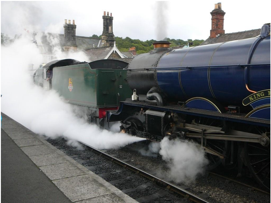
Sorry photographers! - Cylinder drain cocks open, starting from cold – NYMR Steam Gala
