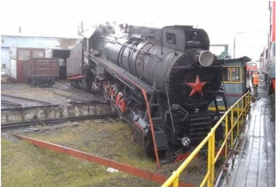
Russian 2-10-0 LV-0123, Perm depot, 12 th October 2019. Loco left “in gear” before fire was lit. Lifted and repaired now. Thanks to Robin Patrick for sending this to ML
